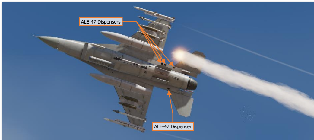
AN/ALE-47 Airborne Countermeasures Dispenser Locations
