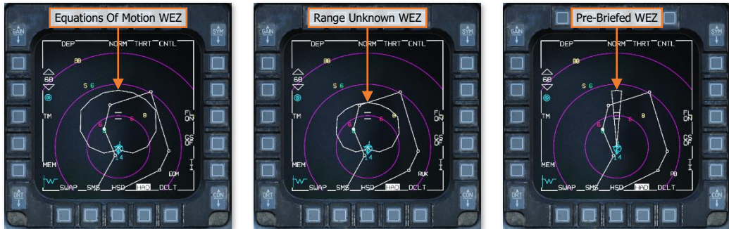
HARM WEZ in EOM (Left), RUK (Center), and PB (Right) launch profiles
