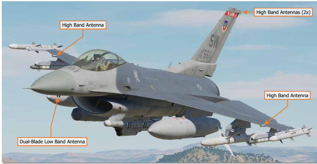
AN/ALR-56M Advanced RWR Antenna Locations
