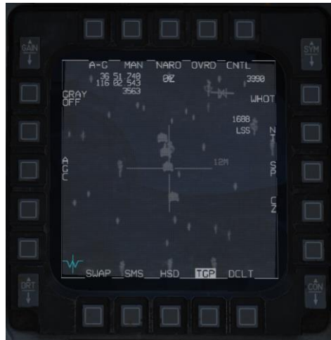
Targeting pod in INR (inertial rates) track mode (crosshair is enlarged)
