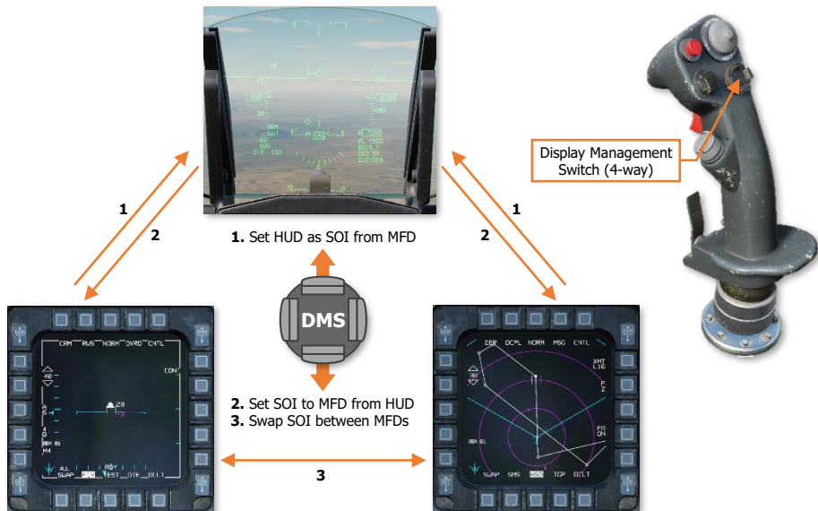
SOI assignment cycle logic using Display Management Switch
